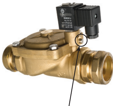
Emergency override manual release grub screw head.
