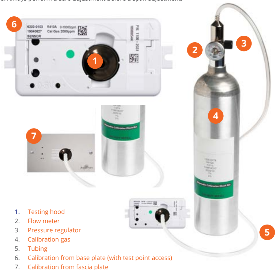
Figure 21. Calibration Assembly
