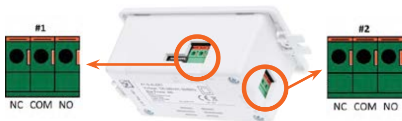
Figure 9. Wiring Relay 1 (Low Gas Alarm) and Relay 2 (High Gas Alarm or Fault)
